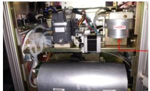
Disassemble the left of the cover , use a small screw driver to fine adjustmentthe bottom of the hole of the PEEP valve's.
