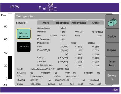
Ambient press. Output of ambient pressure measurement values. Measuring range 600
