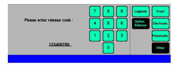
This menu can be used to release software options with a 10-position code. The code number is governed by the ID number of the Evita. Checking is performed after entering the number. If check is positive, software option is ready for use next time the unit is switched on.
