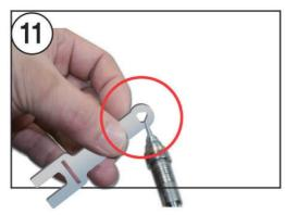
Set the middle part of the wrench on the front of spindle.
