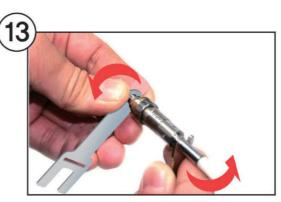
Turn the two wrenches to the arrow direction and loosen the spindle a little.
