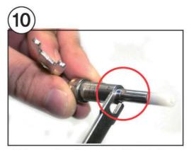
Fit the wrench on the rear part of the spindle.
