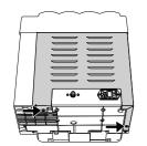
▶ Remove the two Torx 3x10 screws, and remove the rear wall from the device.
