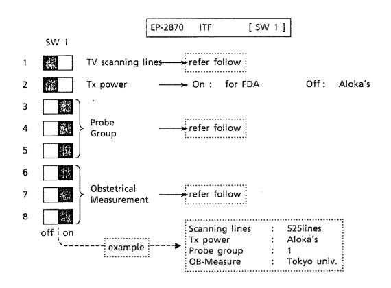
······ On : 625lines TV Scanning Lines Off: Caution : If change the TV scanning lines, it is necessary to replace EP-2871
