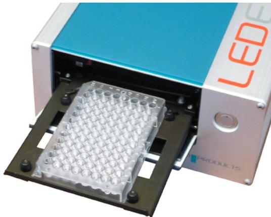
LEDETECT 96 is a computer controlled microplate reader for 96 well plates. Easy and safe operation take away the hassle from your daily microplate reading jobs. It is based on the most modern LED technology, no need to worry about lamp replacements anymore.
