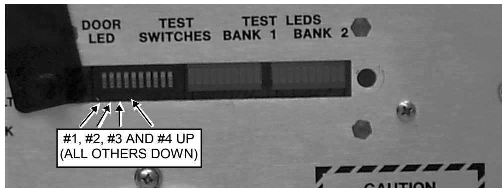
DIP SWITCH CONFIGURATION FOR SETTING POWER MONITOR TYPE ILLUSTRATION 9-1
