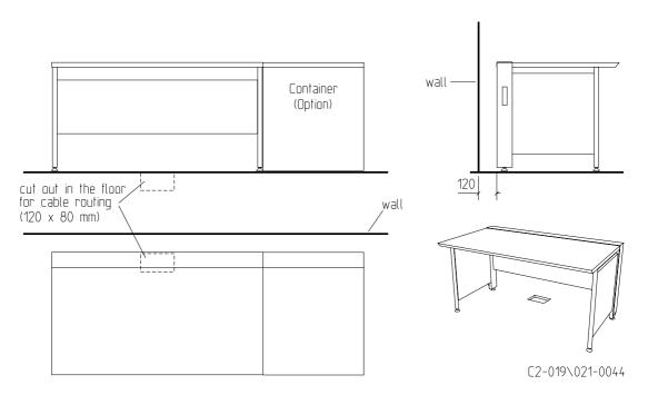
• A distance of 120 mm from the wall must be maintained for routing cables to the monitor and keyboard
