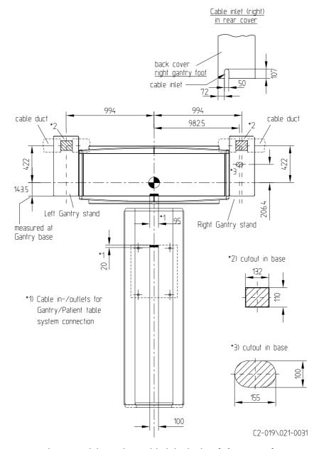
• All cables to the gantry are to be routed through a cable inlet in the **right** gantry foot.
