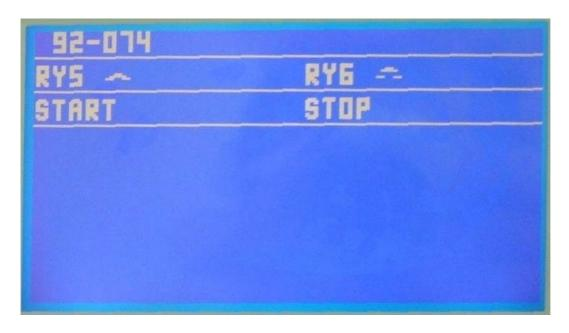
RY5 must be CLOSED for normal operation, if OPEN: Check onboard fuse F3 or flat cable connection to the CPU or RY5 relay and contact.
