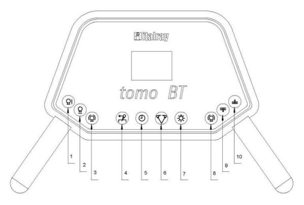
To enter SETUP press at the same time keys 1 and 2.during normal functioning of the equipment.
