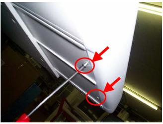
• Remove the fixation nuts from the top panel (4 bots on the external sides for single console; 5 bots for integrate console, 4 on the external sides and one in the center.
