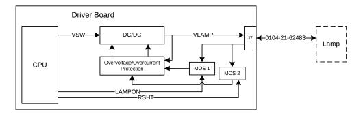
The lamp needs +6V when working and +2V on standby. The voltage is provided by the DC/DC unit, which is controlled by the VSW signal from the CPU and sends VLAMP signal to the lamp. The VLAMP signal also feeds to the overvoltage/overcurrent protection unit, which controls the DC/DC unit to stop power supply to the lamp when overvoltage or overcurrent occurs.
