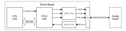
There are three groups of signals to control the analog board: digital potentiometer control signal DCPx, channel gating signal CHx, and AD collection control signals AD\_Ox and AD\_Ix. All signals are generated from CPLD and processed by level translators.
