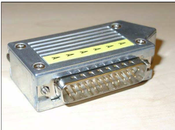
Fig. 1 Bottom view of shield temp adapter
