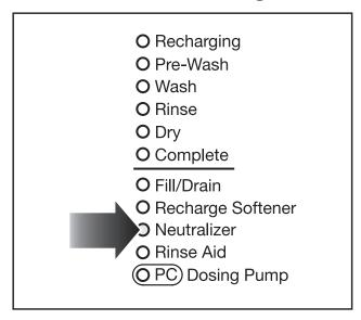
■ When the "Neutralizer" indicator comes on, it is important to promptly refill or exchange the neutralizer container.
