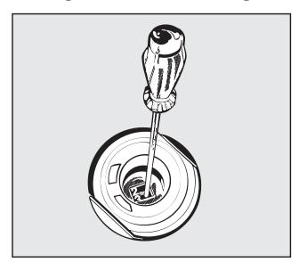
The dosage selector has settings from 1 to 6 (1 - 6 ml). The factory setting is at 3 (3 ml).
