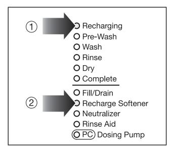
When the salt reservoir is empty, the "Recharge Softener" indicator ② lights to remind you to fill the reservoir.
