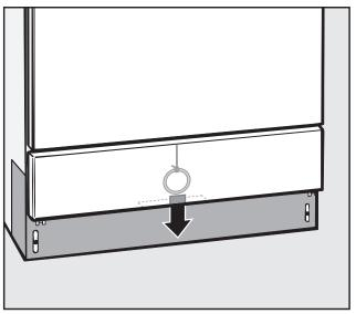
■ Locate the ring for the emergency release cable (at the bottom of the machine, behind the service panel), and pull the ring downward to open the door.
